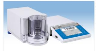
Microbalances MYA 3Y series are intended to measure mass with the highest accuracy. They feature 5,7" LCD colour touch panel which provides new possibilities of balance operation and presenting measurement results. Measurement reliability and accuracy are maintained by system of automatic internal adjustment / calibration.
