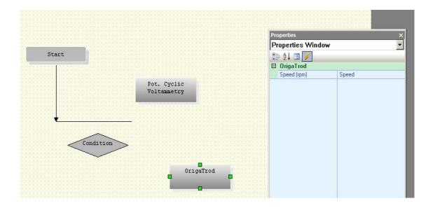
The following sequence contains the "?" block, the conditional block. It allows, depending on the condition, the repetition of a sequence, until that condition is fulfilled.
