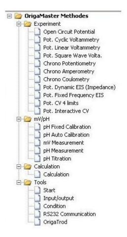
The programming of a method is done with ease : through logical blocks. It is necessary to use a "Start" block, which can then be followed by any sequence of methods requested by the user. Any used block can be renamed and any link between two blocks can get a short annotation. For every block there is a properties window in which you can change the existing parameters.
